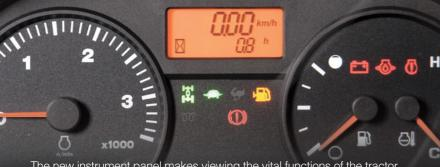
The new instrument panel makes viewing the vital functions of the tractor clear and easy. The LCD readout displays travel speed, PTO revolution and hour meter information digitally. Illuminated analog indicators include a large tachometer, temperature gauge and fuel gauge. A battery warning light has also been added to these tractors to prevent surprise battery failures, as well as indicator lights for 4WD engagement, PTO and oil pressure.
