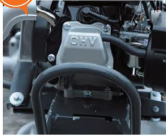
The machine is equipped with powerful OHV gasoline engine with total displacement of 192 cc that allow effectively work at a speed of 0.85 m/s. (10% faster planting speed compared with previous model)
