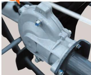
The axle case has been changed from a grease method to an oil bath method to improve maintainability and durability.
