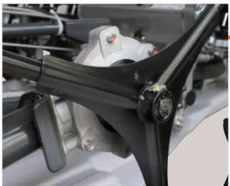
Durability is enhanced thanks to the hexagonal axle which prevents the axle pin from being broken.
