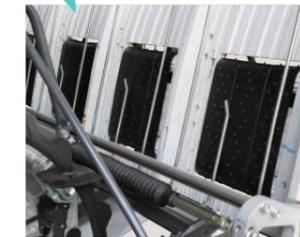
The KW4 is equipped with a belt type vertical feeding mechanism for the seedling tray increasing the holding power of the seedling mat. It can prevent the seedling mat from slipping down enabling more stable planting.
