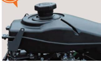
The fuel tank has a large capacity of 10 L (Previous model: 4L). The reduced number of refueling contributes to its efficiency.
