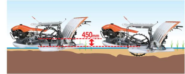
The auto sensor detects undulations to adjust the machine height up to 450mm contributing to efficient operation even in deep paddy fields.
