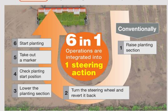
The automatic raise/lower function of the planting section and the line marker operation are seamlessly linked to handle turning. The machine automatically aligns planting with the previous row, making turns in paddy fields more efficient and significantly reducing operator workload.
