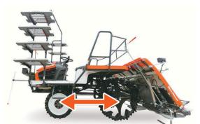
The longer wheelbase enhances machine stability, allowing it to cross ridges and wet field conditions with greater ease.
