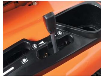
*Hydraulic mower lift lever*
