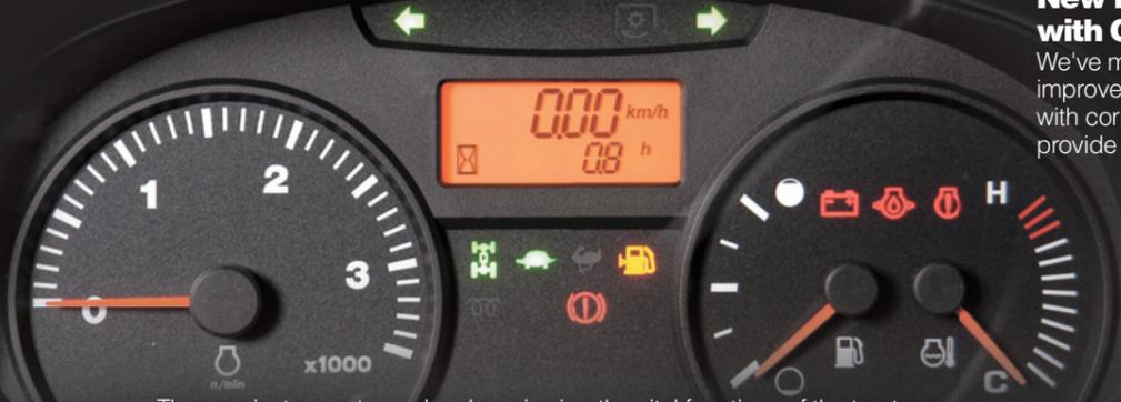
The new instrument panel makes viewing the vital functions of the tractor clear and easy. The LCD readout displays travel speed, PTO revolution and hour meter information digitally. Illuminated analog indicators include a large tachometer, temperature gauge and fuel gauge. A battery warning light has also been added to these tractors to prevent surprise battery failures, as well as indicator lights for 4WD engagement, PTO and oil pressure.
