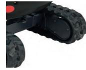
Travel motor hoses are enclosed within the track frame for additional protection.
