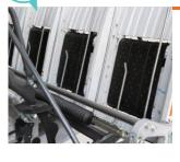
The KW4 is equipped with a belt type vertical feeding mechanism for the seedling tray increasing the holding power of the seedling mat. It can prevent the seedling mat from slipping down enabling more stable planting.
