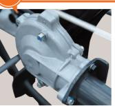
The axle case has been changed from a grease method to an oil bath method to improve maintainability and durability.
