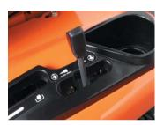
Hydraulic mower lift lever
